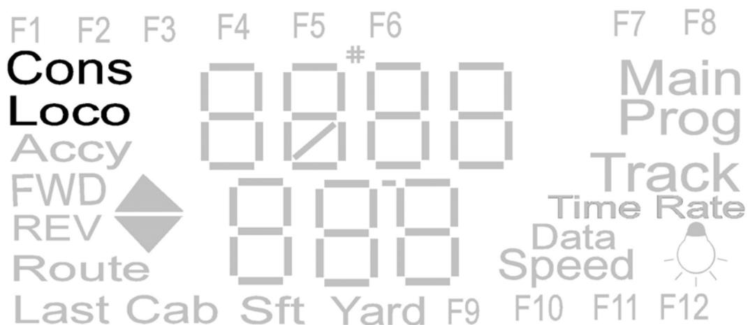
The MAIN / PROG / TRACK and DATA icons are displayed in programming and (READ) modes, the SFT (shift) icon is used in function selection and when selecting in READ mode
