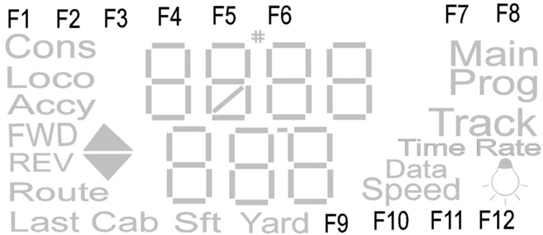
FWD / REV and SPEED icons display the loco speed and direction of travel
