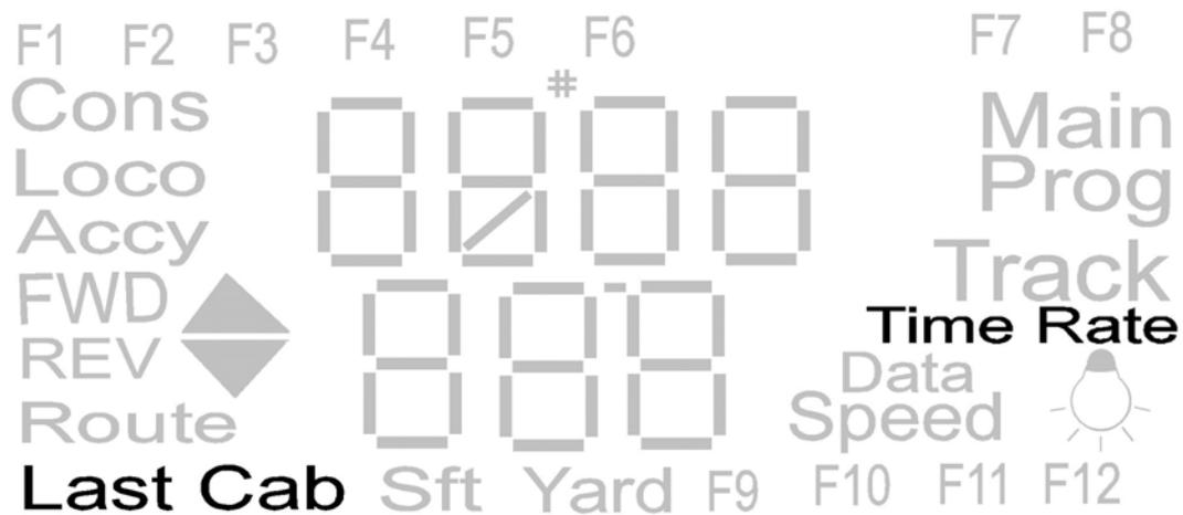
The LOCO and CONS icons are displayed when operating and programming locomotives and consists (DBL HEAD)
