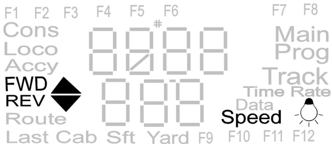
The LAST CAB icon is used in the system setting and the TIME RATE icon is displayed when operating the (fast clock) time mode
