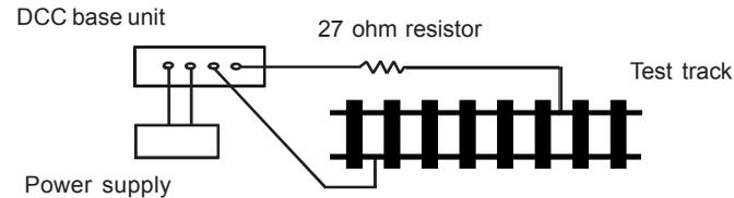
Fig3. Diagram of test track
