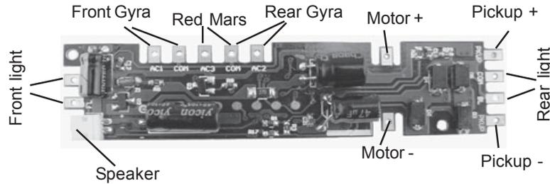
Figure 1 shows the connections to the decoder board.
