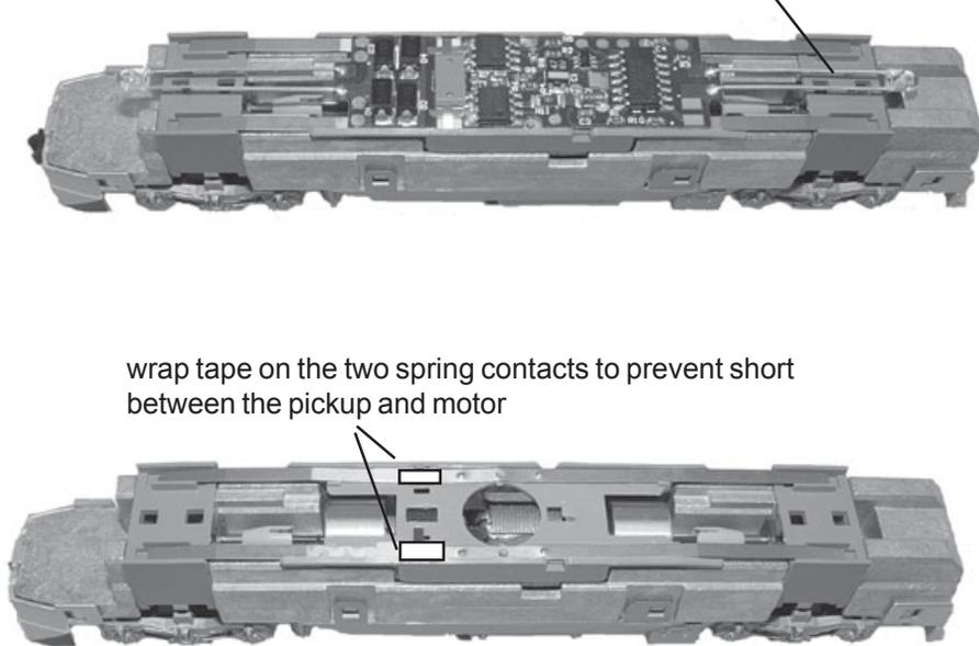
Figure 2: Kato Chassis after removing original circuit board
